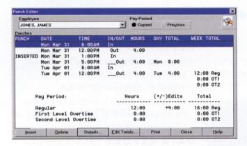
Punches which are edited using the PC Interface are tagged and stored in the database.
