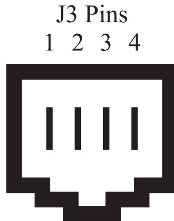
Figure 4-2: J3 - RJ-11/RS-422 Jack Pinout
