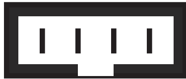
Figure 4-2: J4 - RS-232 Jack Pinout
